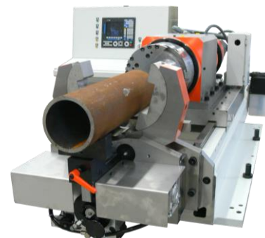
Facing – Chamfering – Beveling – Threading – Grooving – OD & ID Turning of any Contours
