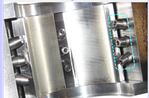
5 Pad Bearing 3 lubricant feed nozzles per pad
